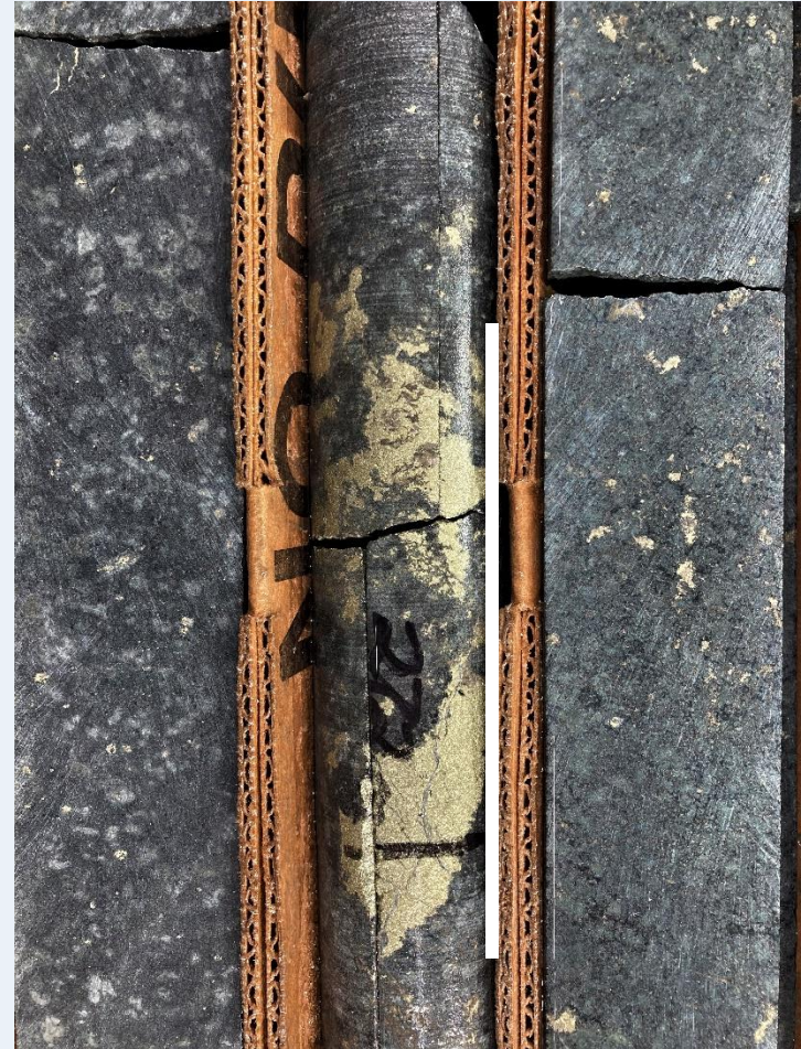
Rip-up Clast grades 7.13% Ni, 7.91% Cu over 8 cm sample
