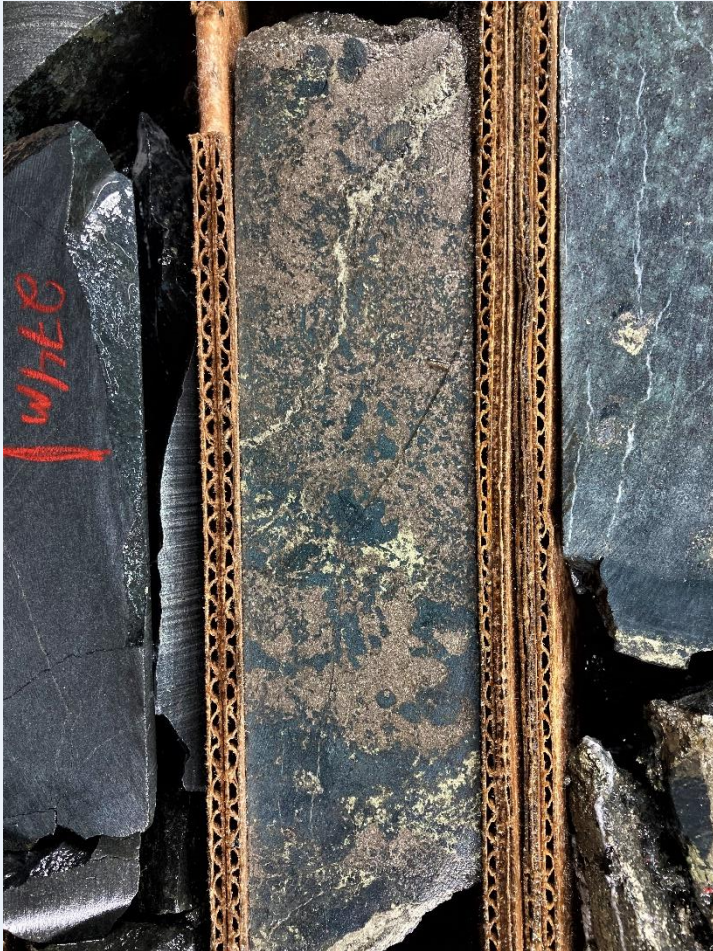
Semi-Massive mineralization grades 5.16% Ni, 1.18% Cu over 0.75 metres
