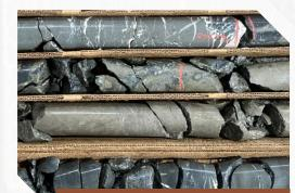
80 cm of massive sulphide at base of LM-21-14
