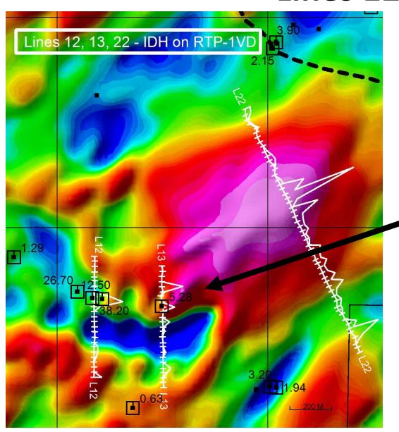
Soil IDH response with high-grade Gold on the margins of the Line 22 intrusion (?) as per Sillitoe's model
